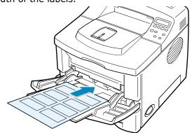
3 When you print on labels, configure the paper source, type and size properly in the software application. For details, see page 5.7.
